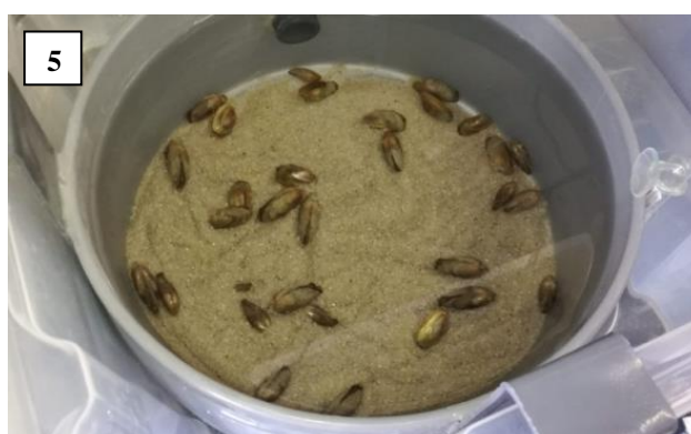
Figure 4. General setup of the experiment. See water tank with PVC cylinder holding inside, with a water pump connected and naiads waiting for the inoculation process in plastic boxes. Figure 5. Closed details of the experiment. PVC cylinder with silica sand sediment at the bottom and settled naiads. The PVC cylinder is holding from the plastic tank. Because it is semi-floating and has a grid bottom, water can recirculate from the outer to the inner part of the cylinder thanks to the water pump.
