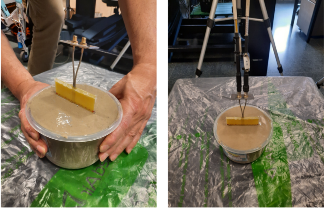
Figure 45: Antenna embedded in cement.
