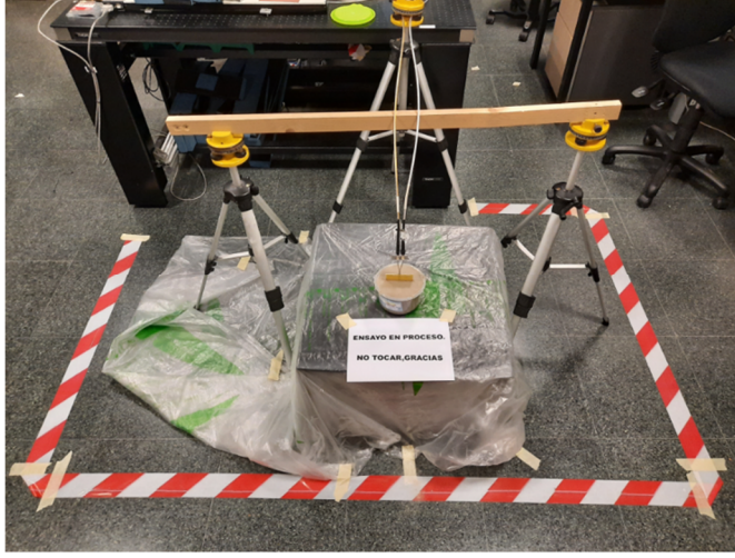
Figure 46: Scenario to measure the antenna in cement.
