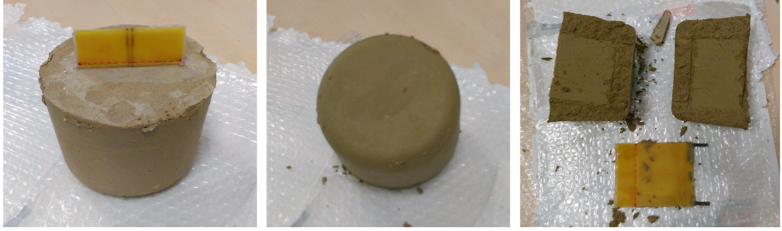
Figure 48: State of the cement after 24 h – Antenna removal.
