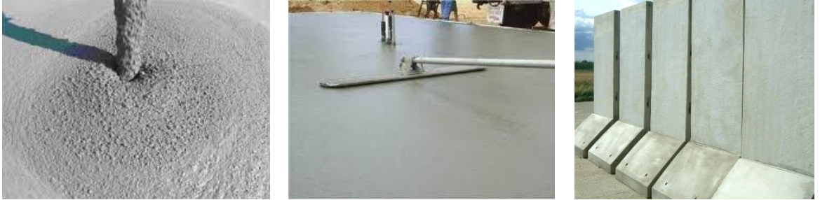
Figure 6: Concrete in fresh state, setting state and hardened state respectively.
