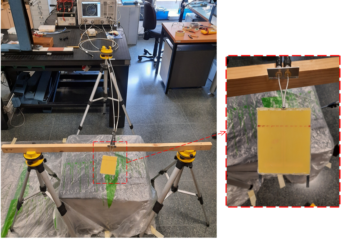
Figure 42: Scenario to measure the antenna in free space with both FR4 plates sealed.
