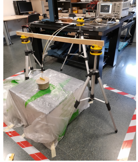
Figure 46: Scenario to measure the antenna in cement.
