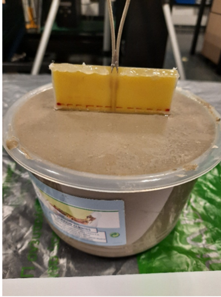
Figure 47: Antenna embedded in cement after 9 h together with FEKO design for comparison.
