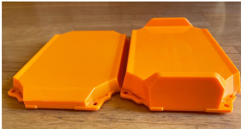
Figure 3.12: Sensor case "Rubicon" tapes size comparison. left: latter units tape, right: first unit tape.
