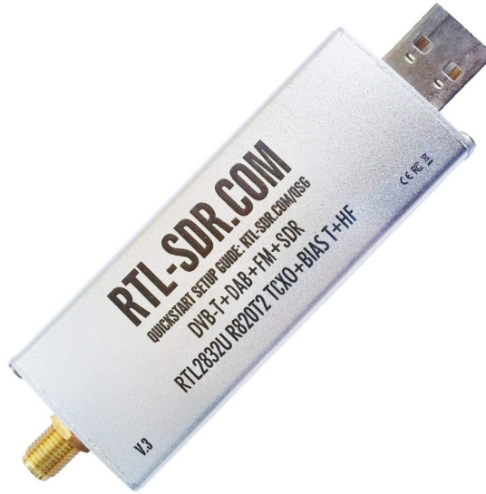
Figure 3.5: RTL-SDRv3 RF front-end.
