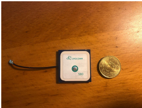
(a) A Cirocomm 580R antenna near a 10 euro cents coin. Top view.
