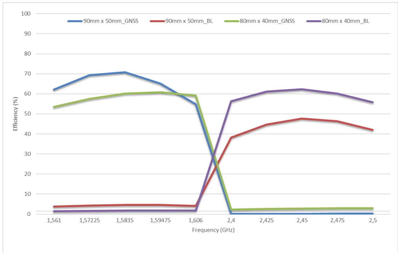
Figure 63: 90x50mm vs 80x40mm Full Layout efficiencies antenna in the middle
