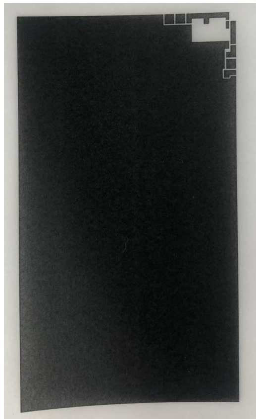
Figure 65: Mask used for the experiment of the DUO mXTENDTM in the corner in a 90mm x 50mm PCB
