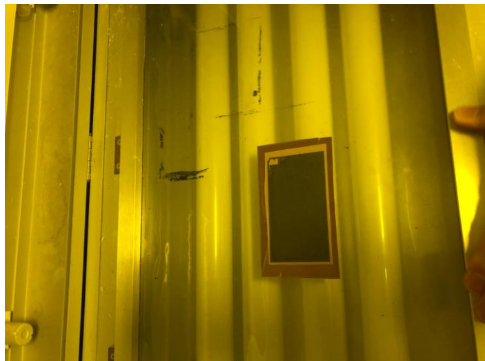
Figure 67: The UV contact printer with the footprint mask done right above the board
