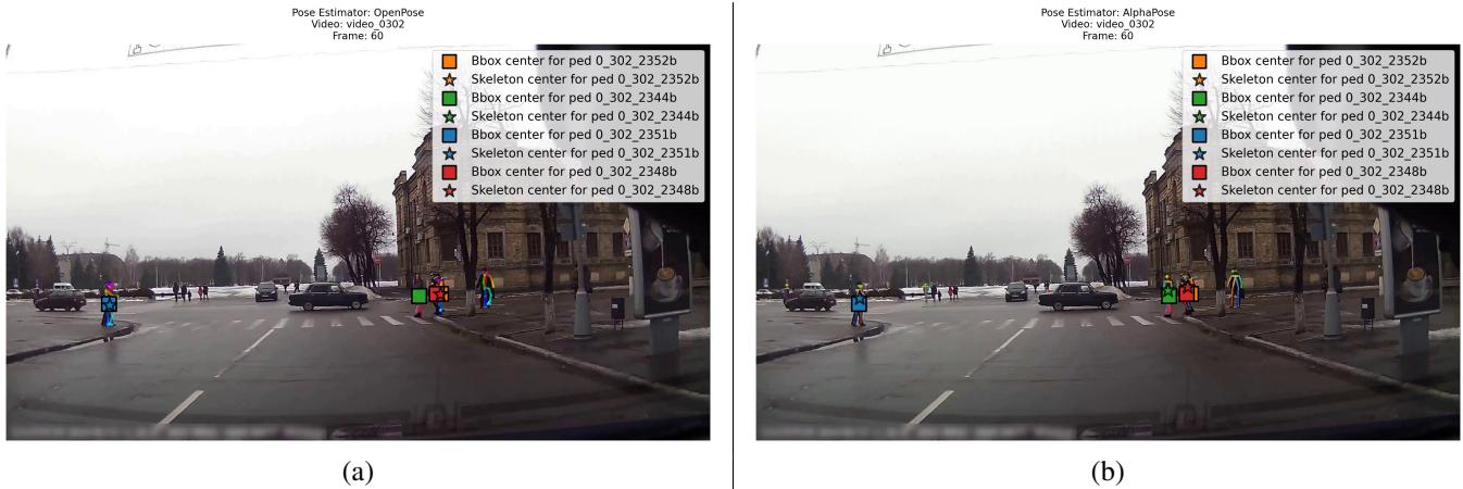
Fig. 13: Center of the bounding boxes and the estimated skeletons of the pedestrians appearing in frame 60 of JAAD video 302: (a) Using OpenPose skeletons; (b) Using AlphaPose skeletons
