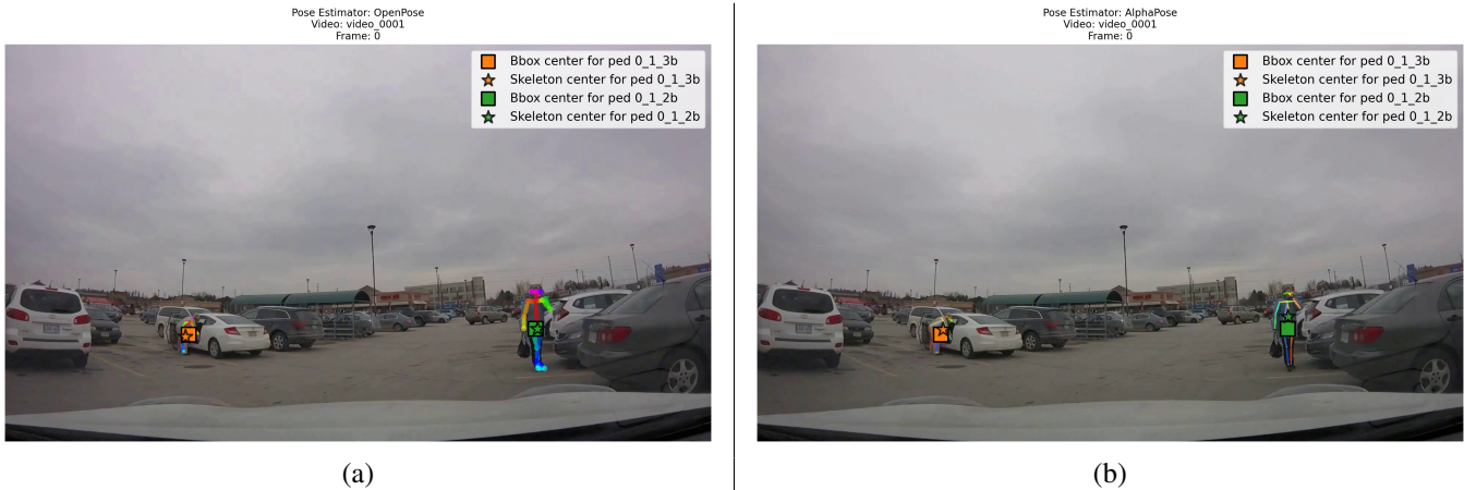
Fig. 12: Center of the bounding boxes and the estimated skeletons of the pedestrians appearing in frame 0 of JAAD video 1: (a) Using OpenPose skeletons; (b) Using AlphaPose skeletons
