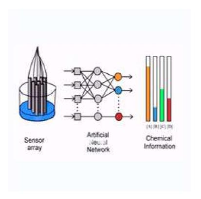
Electronic tongues are analytical systems which are used to recognise the chemical components in a liquid. For these systems to be able to decode information they need the aid of computers and applied artificial intelligence tools. In his doctoral thesis the researcher Jordi Gallardo Oña has developed a procedure which allows for the design, construction and evaluation of an electronic tongue.
