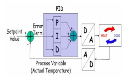
A simple negative feedback control loop makes the process variable close to the set-point even if there are disturbances. The common strategy is to develop a mathematical model of the process and, based on it, to select appropriate values for the control algorithm parameters. In contrast with many empirical methods, this communication proposes the analytical tuning of a commercial PID controller based on a FOPDT model. The objective is to obtain smooth responses.
