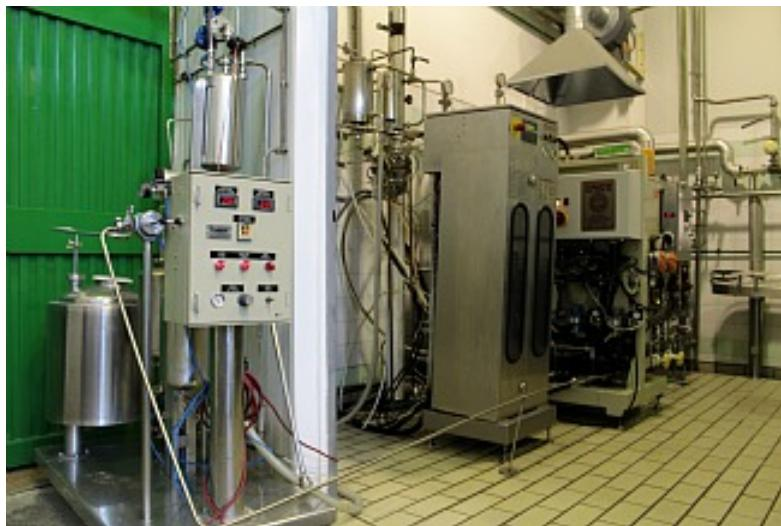
The UAB Food Technology Plant Special Research Centre (CERPTA) has designed a new system capable of sterilising and stabilising liquids at high pressure, thus allowing them to last longer at room temperature and reduce the use of additives to preserve organoleptic qualities. The technology also protects the bioactive components of foods. To commercialise the product, CERPTA and UAB created YPSICON, a technology based spin-off company.
