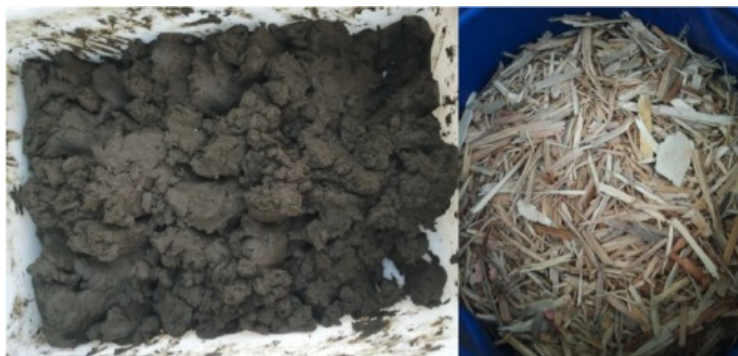
Figure 1: Raw sludge and shredded pallet (bulking agent) before being mixed in an adequate ratio for composting treatment.
