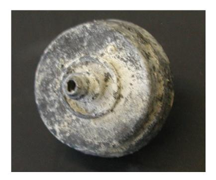
Drip irrigation optimises water reuse and makes irrigation more efficient, but the system often presents problems of obstruction caused mainly by the accumulation of material of biological origin, which often begins with bacterial biofilms. A study of biofilms clogging the irrigation system of an experimental greenhouse in Almeria has found a predominance of microorganism sequences adapted to growing in environments with high temperatures related to potential spore-forming organisms.
