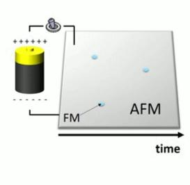
Sketch of the transition between antiferromagnetic (AFM) and ferromagnetic (FM) states depending on the applied electric voltage.
