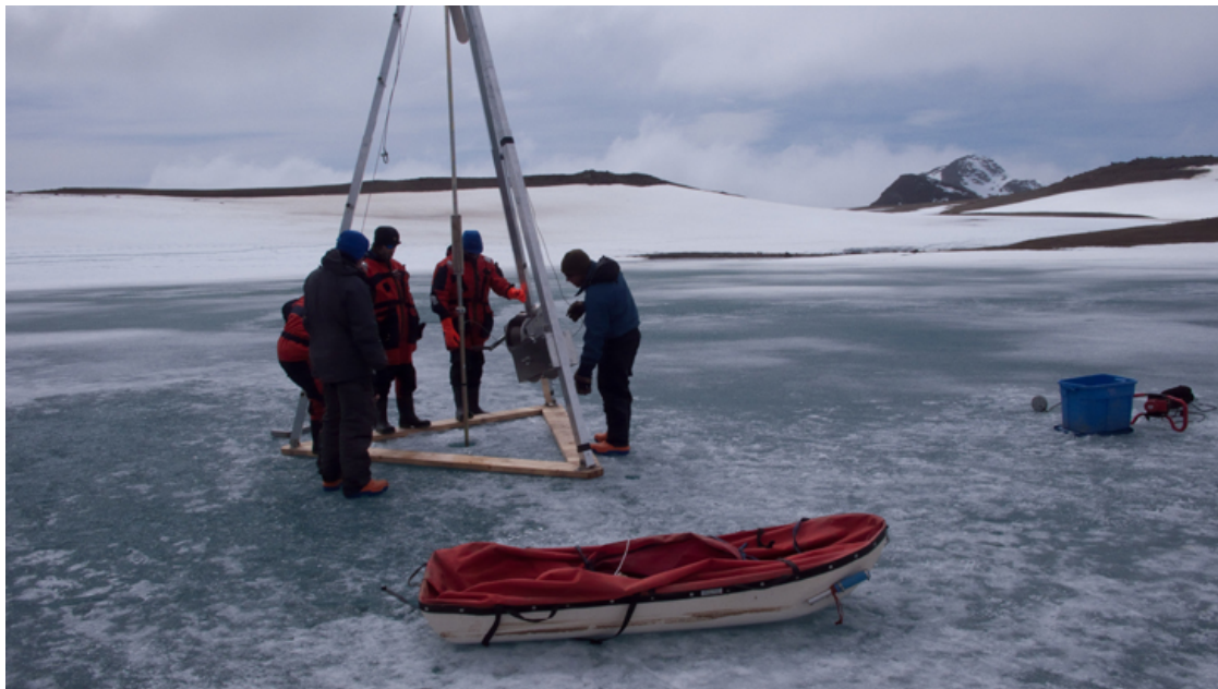
The research team extracting records to date the eruption of the volcano thanks to the ice drilling platform. Photography by Sergi Pla Rabès.
