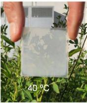
The Department of Chemistry of the UAB in collaboration with the ICN2 have developed a new class of smart windows of low cost and facile fabrication based on polymeric coatings loaded with organic wax nanoparticles. Thus, at low ambient temperatures or with little solar radiation, the window is transparent and at high temperatures or on sunny days it turns opaque.
