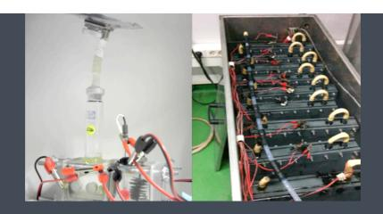
The GENOCOV research group investigates microbial electrolysis cells, systems that treat wastewater while generating resources. One of the key practical aspects in the performance and feasibility of these systems is the cathode material, where hydrogen is generated. In this study, they have tested nickel foam as a cathode for the first time and have achieved the highest hydrogen production ever recorded on a pilot scale.
