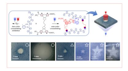
The lithographic and 3D printing techniques are limited by long printing times or low resolution, which prevents reaching micrometric scales. The Department of Chemistry takes part in the development of an alternative technique: polymer photocuring. This process enables the control of polymer formation through light irradiation to produce solid materials more quickly and with higher resolution.
