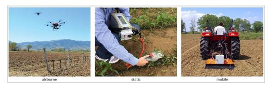
Figure 8: Measuring soil and crops. Soil and crop vis-NIR spectra are measured at points or by imaging from various developed platforms by i-BEC
